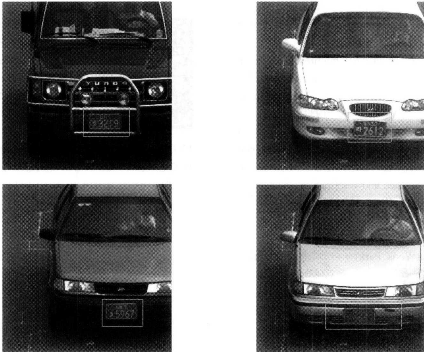
Fig. 8 Represents the result of mapping coordinates of plate region determined in (d) of Fig. 7 into vehicle image
