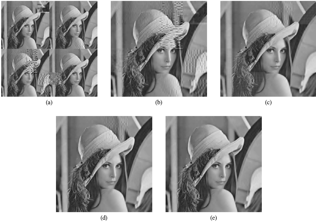
Fig. 7 Lena image decoded with different ways. (a) Corrupted subsampled image; (b) Corrupted represented image; (c) Zero-replacement; (d) MREC-BS; (e) MREC-ES
