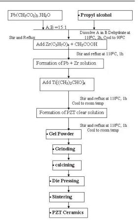
Fig. 1. Flow diagram for the preparation of PZT
