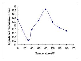
Fig. 5. Impedance resonance as a function of temperature
