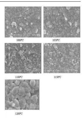
Fig. 3 SEM morphology of PZT ceramic calcined at 9000C for 4h and sintered at  $1000\,^\circ$ C,  $1050\,^\circ$ C,  $1100\,^\circ$ C,  $1150\,^\circ$ C,  $1200\,^\circ$ C for 2h
