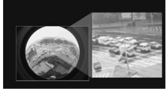
Fig.2. The blurring is occurred because small size image of fisheye view is spread out to larger size of de-warped image
