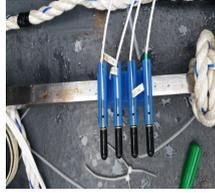
(a) Transducer(ITC-1007)&Transmitting voltage response
