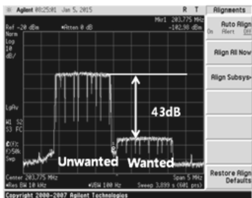
Spectrum analyzer, Center frequency 203.775MHz, span 5MHz, RBW 10kHz Wanted 204.64MHz, -70dBm, Unwanted 202.928MHz, -27dBm
