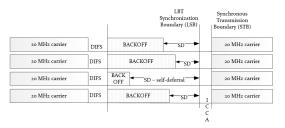
(b) LBT Type A with self-deferral to combat RF leakage
