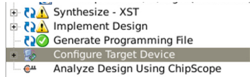
Fig. 13. FPGA Implementation Sequence
