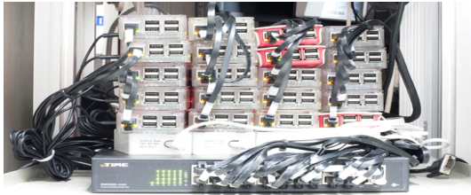
RaspberryPi-based HD-EMA testbed IP address: 192.168.1.41~60
