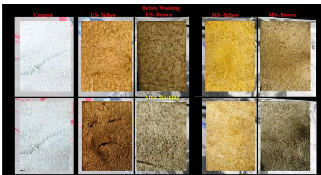
Figure 4. Leather dyed with C. tinctoria yellow and brown dyes. Left: control, with ultrasound yellow and brown; right: with magnetic stirring yellow and brown.
